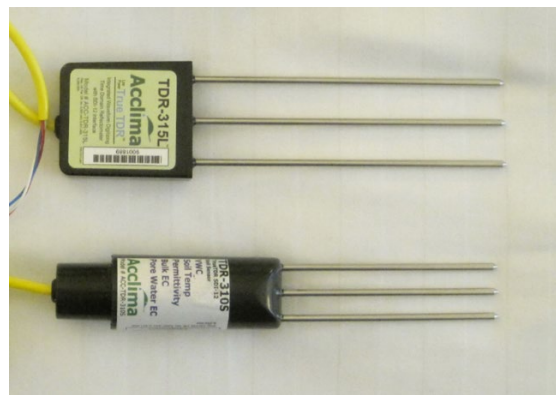
Figure 4. Acclima model TDR-315L (top) and model TDR-310S (bottom) sensors for soil apparent permittivity, bulk electrical conductivity, temperature and volumetric water content.
