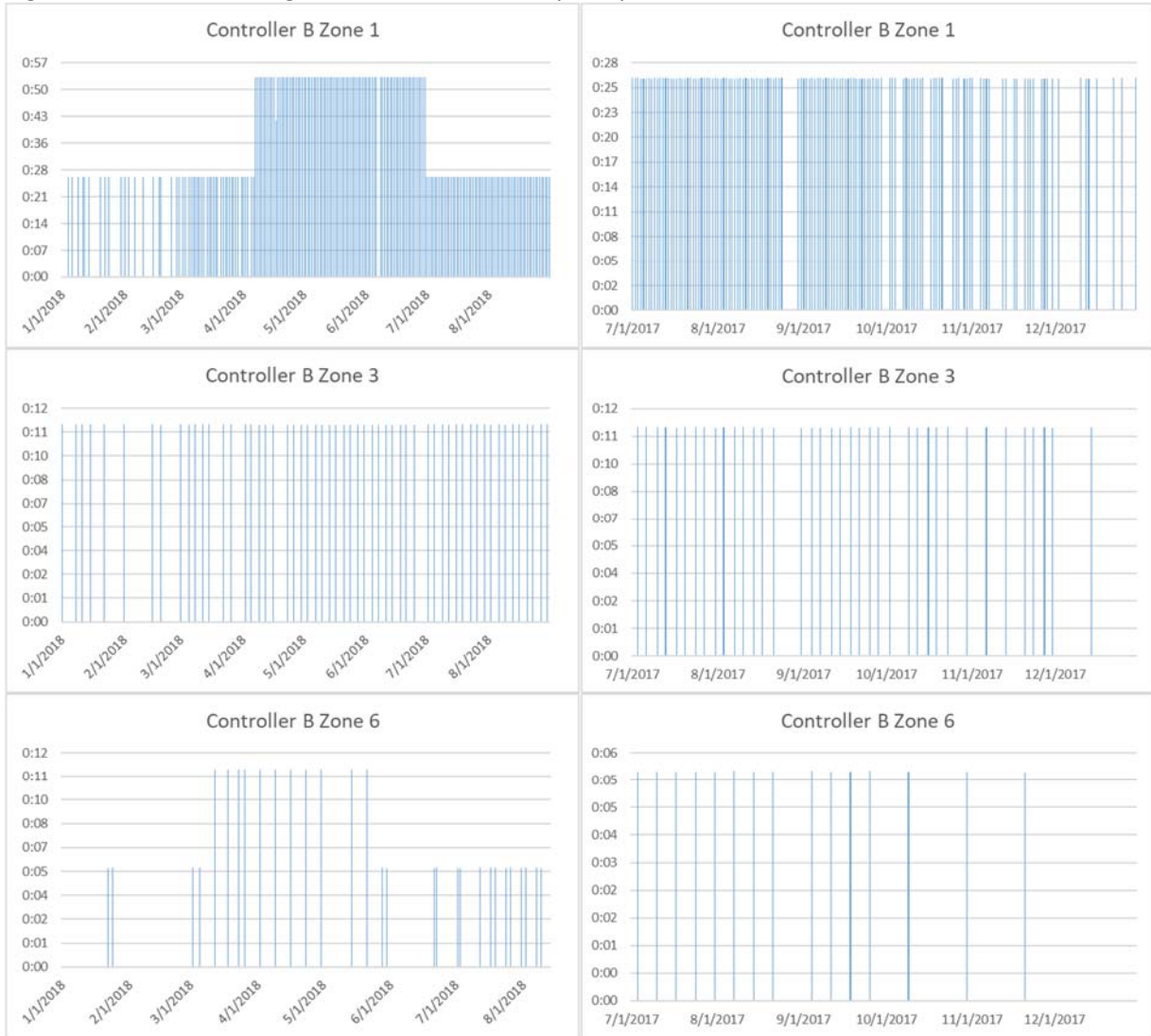
Figure 7. Controller B Irrigation Runtime and Frequency
