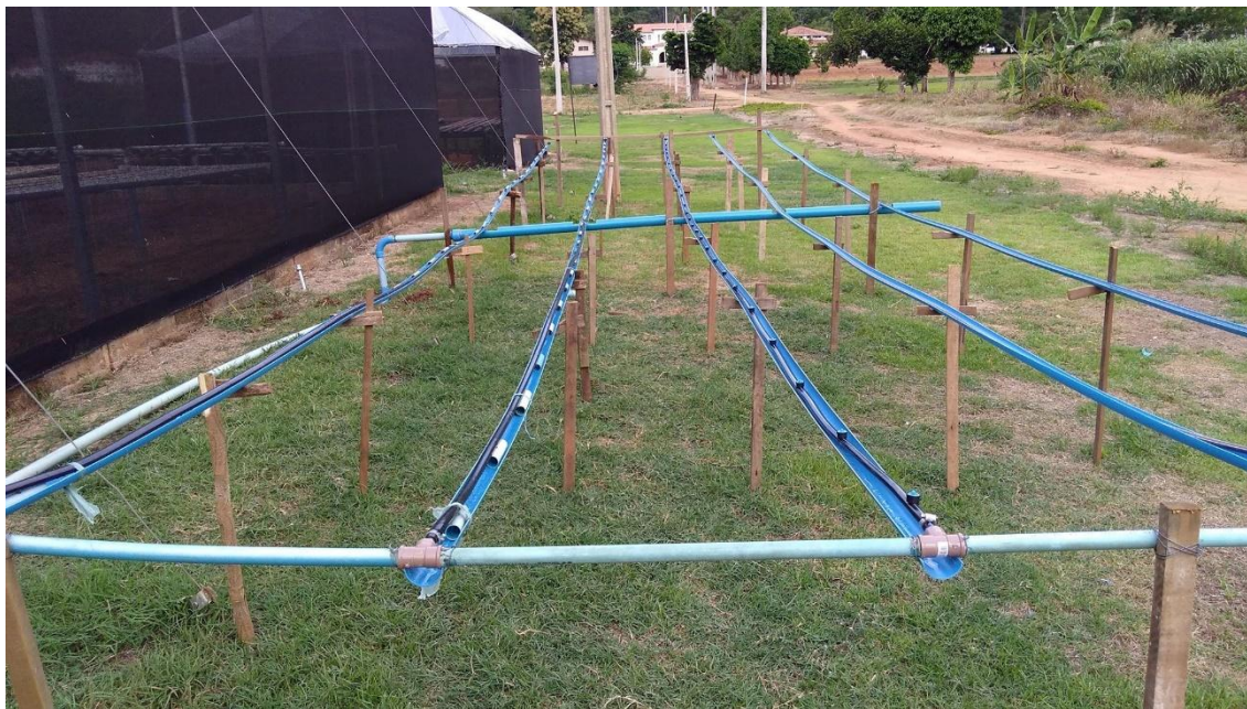
Figure 2. Tests bench for application of treatments and emitters evaluation.
