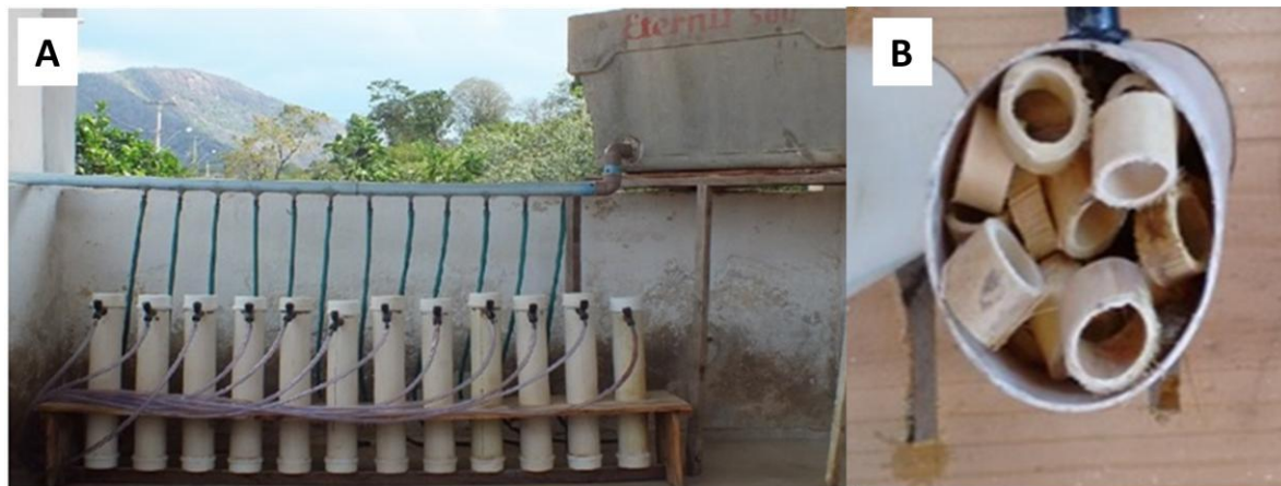
Figure 1. Effluent storage, distribution and filtration structure (A) and top view of the filter showing the filter material (B).
