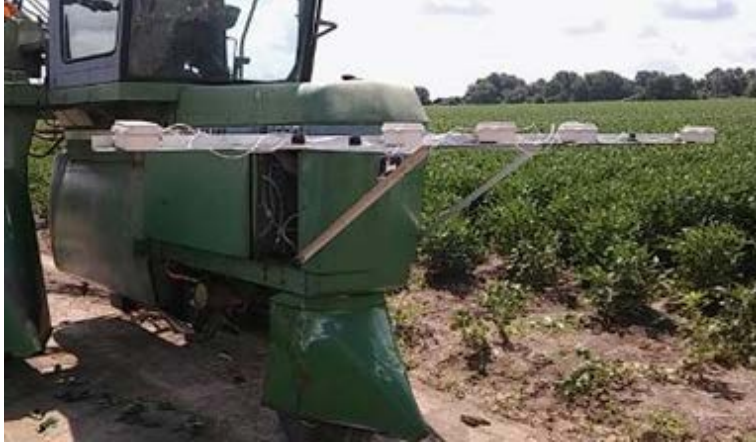
Figure 5. Complete plant canopy monitoring system mounted on an agricultural vehicle.
