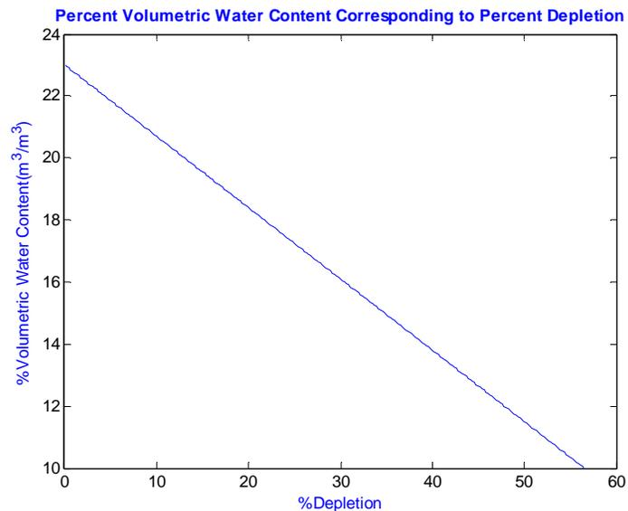
**Fig 5: MATLAB Simulation of Changes in Percent Volumetric Water Content Corresponding To Percent Depletion for Sandy Loam Soil with Field Capacity of 0.23 (23%VWC)**
