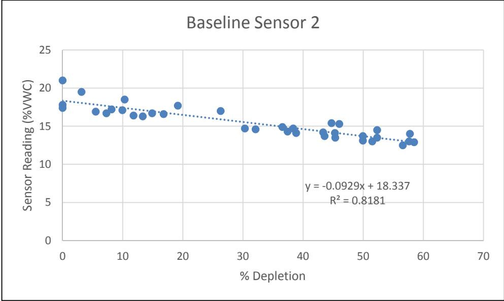
**Fig 14: Repeatability Test for Baseline’s Sensor#2 Over All three Test Cycles**
