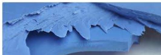
Figure 2 - Layered Structure of PVC
