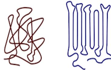
Figure 1 - Amorphous and Semi-Crystalline structures
