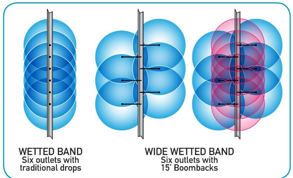
Boombacks, sometimes called offset booms, are add-on accessories for Pivots or Linears to re-locate or offset the sprinkler 15' away from the center line of the span.
