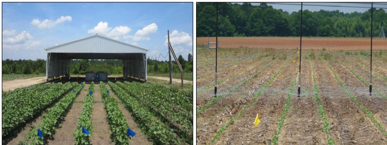
Figure 1. View of the rainout shelter plots (left) and the linear move system with LEPA (right)
