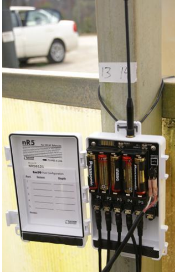
Figure 7. An nR5 node used as part of our wireless sensor network. Up to five sensors can be plugged into the ports at the bottom. On the right side there is a relay that can be used to open and close irrigation valves (red and white wire). The nodes transmit all collected data to a base station and computer using a radio signal.
