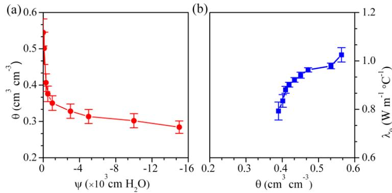
**Fig. 1.** (a) Water retention curve of the soil-mix ( $\theta$  = volumetric water content and  $\psi$  = pressure head), and (b) thermal conductivity ( $\lambda_0$ ) of the soil-mix as a function of the  $\theta$ .
