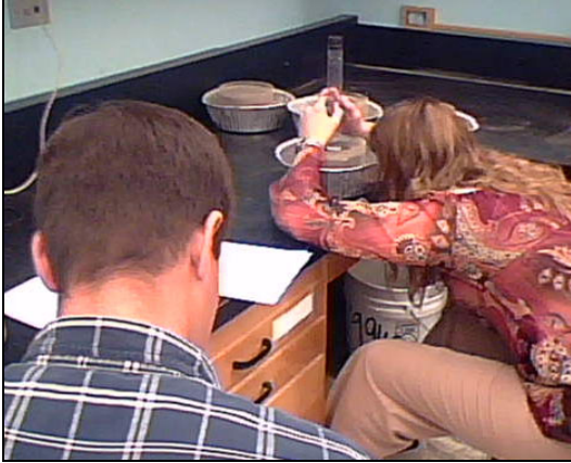
Figure 4. One researcher reads the water level on the mini-disk infiltrometer in the hydraulic conductivity experiment, while another records the readings at regular time intervals.
