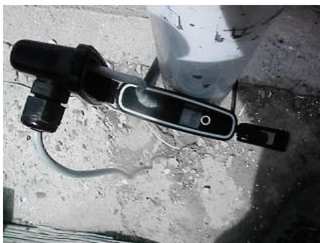
Fig. 2 Irrigation event data logger.
