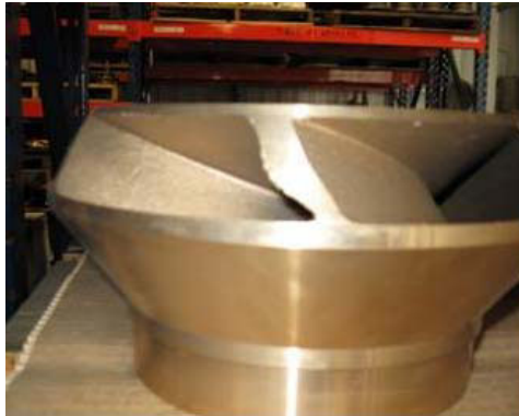
Figure 4. The thickness on the bottom of the vane is correct; the thickness must be reduced on the upper portion of the vane.
