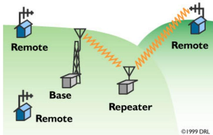
This type of repeating is called 'store and forward.' It is differentiated from full duplex repeating that performs simultaneous reception and transmission, and requires two radio channels. 'Store and forward' repeating is very common in SCADA system design
