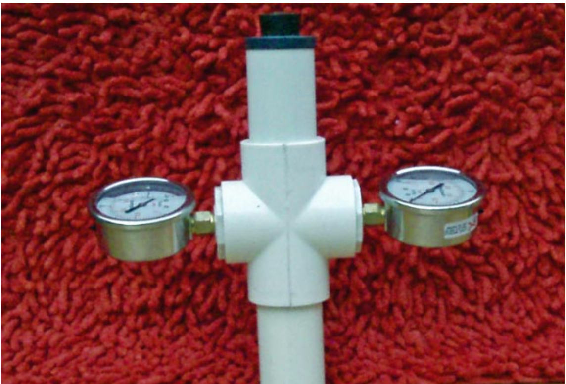
Figure 6: Double ceramic tensiometer. The independent vacuum gauges present information from two independent coaxial porous ceramics.
