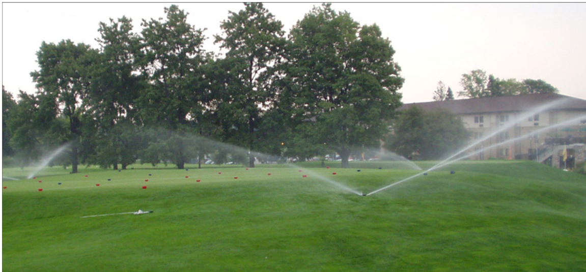
Figure 2. Sprinklers in operation during audit
