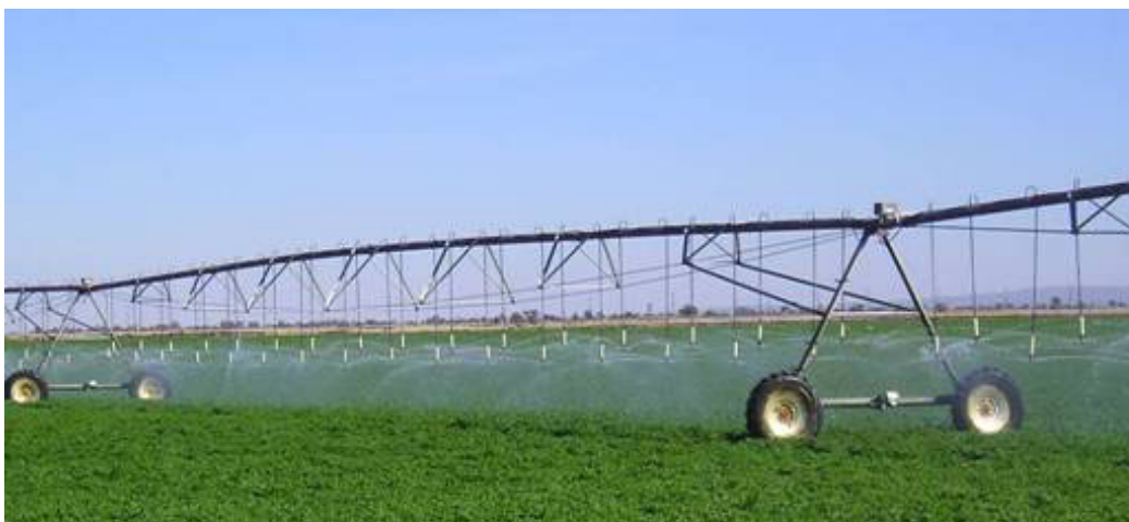
Figure 5. New sprinkler heights – average 5.5 feet
