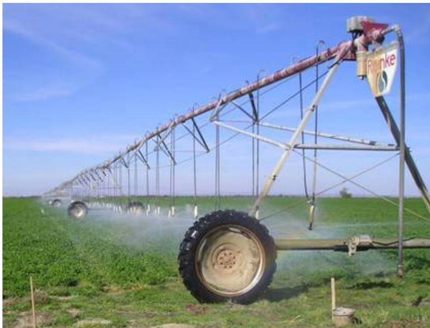
Figure 4. Original sprinkler heights – average 3.5 feet
