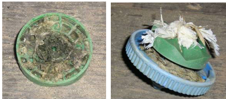
Figure 8. Sprinklers with trash on rotator plates
