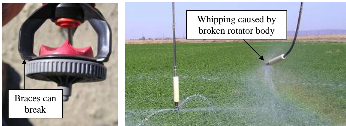
Figure 10. Non-functioning sprinkler because of broken rotator body
