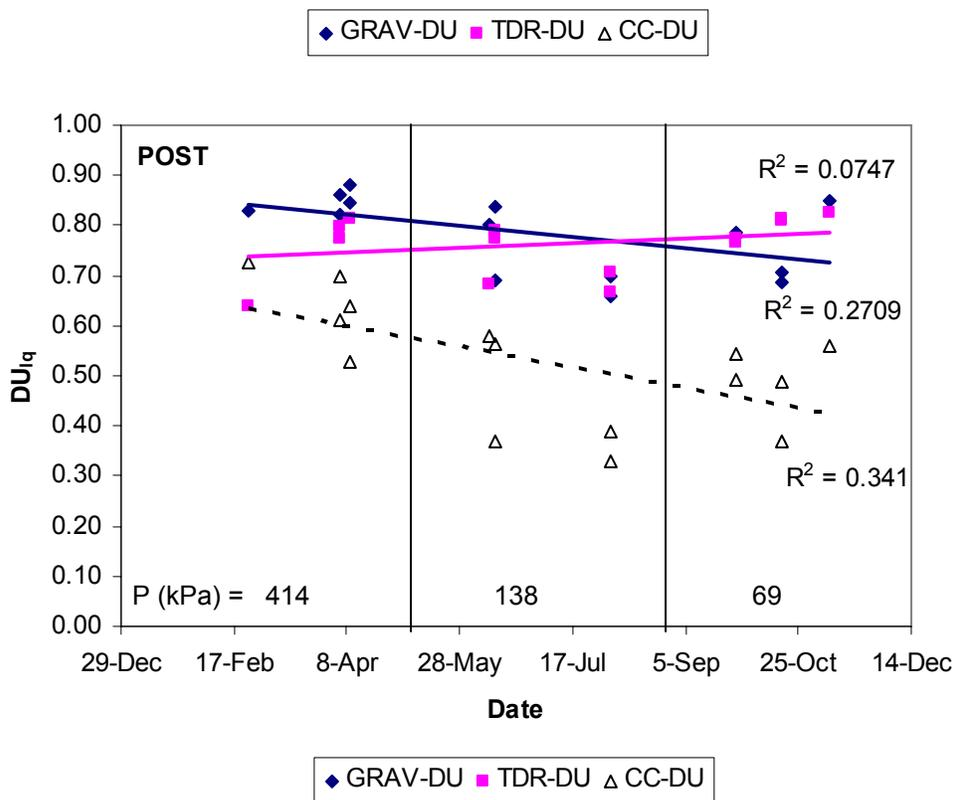
Figure 1. Gravimetric (GRAV-DU), TDR (TDR-DU) soil moisture  $DU_{lq}$  and catch can (CC-DU)  $DU_{lq}$  pre-irrigation and post-irrigation as a function of irrigation system pressure.
