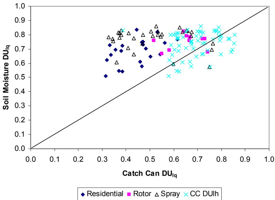
Figure 6. Soil moisture distribution uniformity ( $DU_{lq}$ ) compared to catch can  $DU_{lq}$  for residential, rotary sprinkler, and spray head tests on turfgrass. Note that all soil moisture  $DU_{lq}$  data are also plotted against calculated  $DU_{lh}$ .
