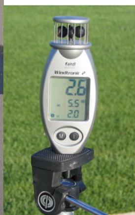
Technicians Rachel Waite and Tessa Berry gather data. A Windtronic anemometer is used to monitor wind speed during the test. It will show current speed, average wind and maximum gust during the test time. Most tests were done with an average wind speed less than three miles per hour to minimize the impact of wind on readings.
