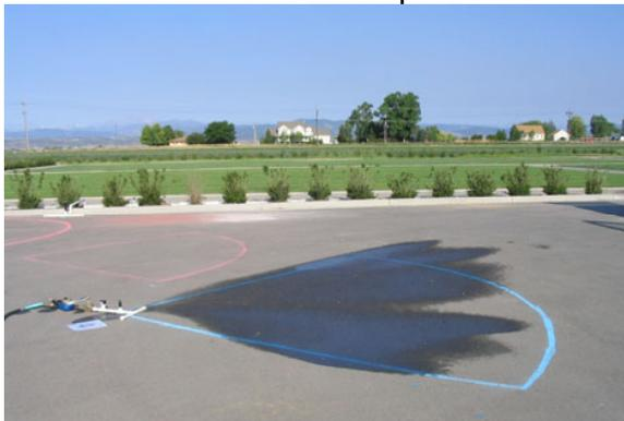
Photographs of nozzles that were tested on the asphalt pad. The photos show more than can be explained even by a catch can test.
