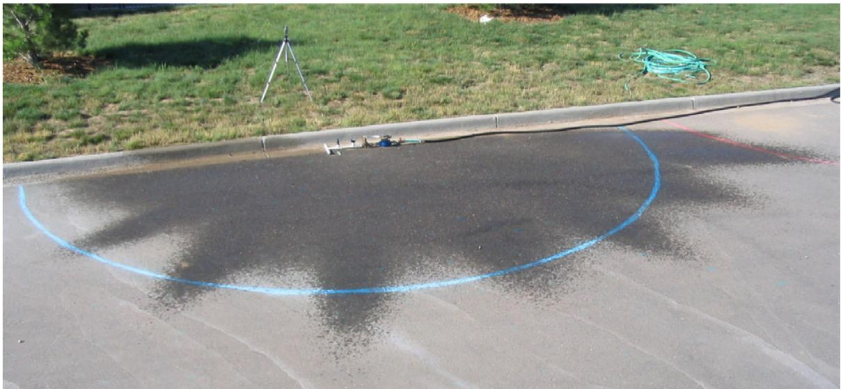
Nozzles are not manufactured equally, and most likely one batch of nozzles will not perform exactly the same as another because of molding issues. The challenge is to understand how they perform individually and then compensate for individual performance when put together in a sprinkler zone. A few of the nozzles had excellent coverage for the pattern intended, but most were not as good as would have been expected.
