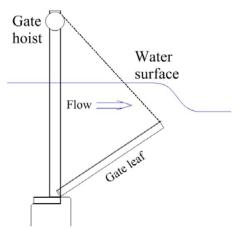
The classical canal overshot gate has a gate-leaf horizontally hinged near the bottom of the canal, with the gate-leaf extending downstream. Water flows over the gate-leaf, which acts as a horizontal weir. The gate actuator is a hoist mechanism that moves the downstream end of the leaf up and down, or in some designs an air bladder under the leaf is used to move the leaf.
