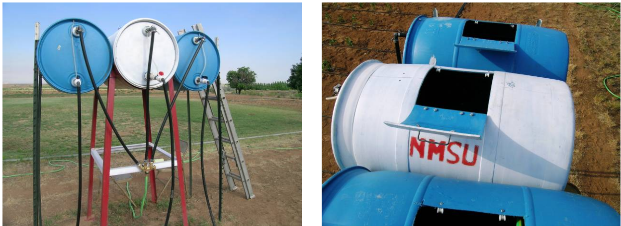
Figure 3. Elevated reservoirs (left) and access doors (right.)
