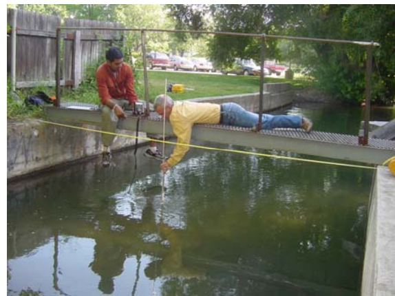
Fig 11. Current metering to check the calibration of a broad-crested weir
