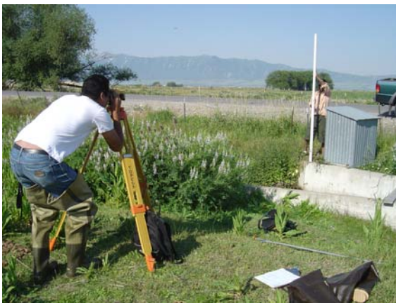
Fig 10. Taking measurements to check the calibration of a flume
