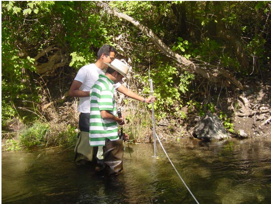
Fig. 9. Current metering in a canal to determine seepage losses
