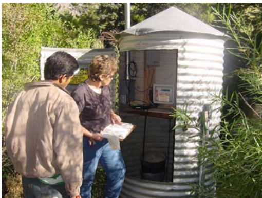
Fig 7. Colleen Gnehm with one of the authors, checking a water level recorder
