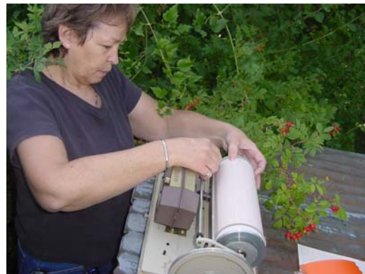
Fig 8. Colleen Gnehm replacing the graph sheet for a water level recorder
