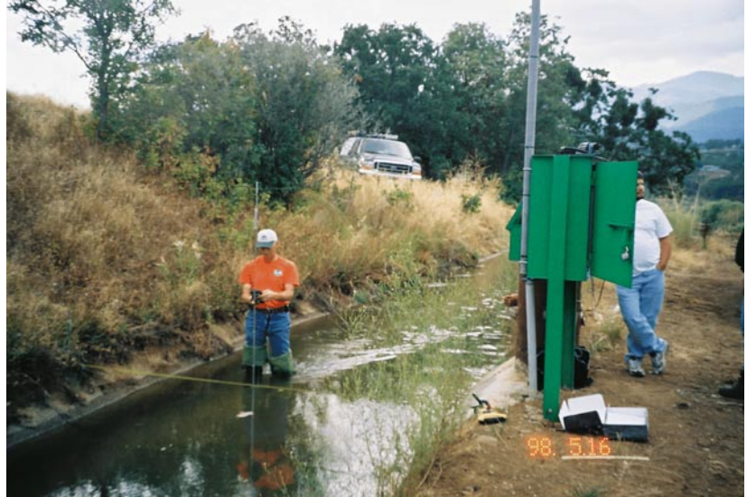
Photograph 3. At the Talent Canal site current-meter measurements were made to provide data which were used to calibrate the velocity readings from the StarFlow instrument. Calibration was required at each demonstration site.
