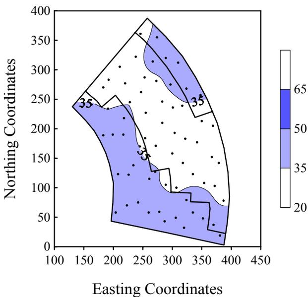
Figure 4. Soil electrical conductivity at one-meter depth used to determine management zones for VR cotton irrigation, 2002.
