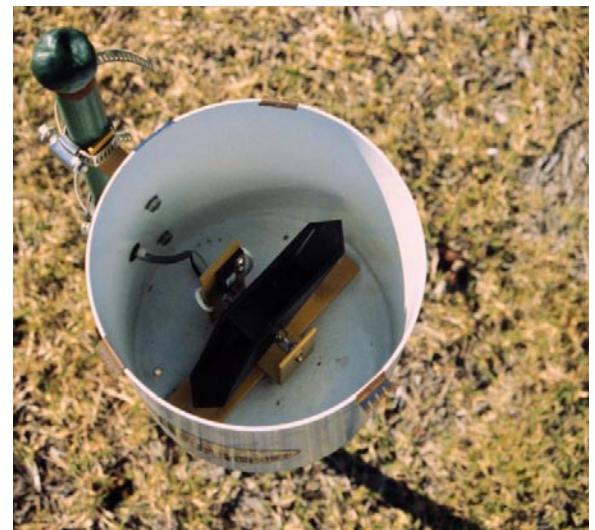
Figure 3. Tipping bucket rain gauge.
