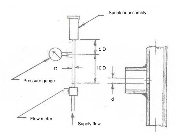
Figure 2. Pressure tap pipe. Note: D refers to pipe internal diameter; d = 1/8 in. diameter
