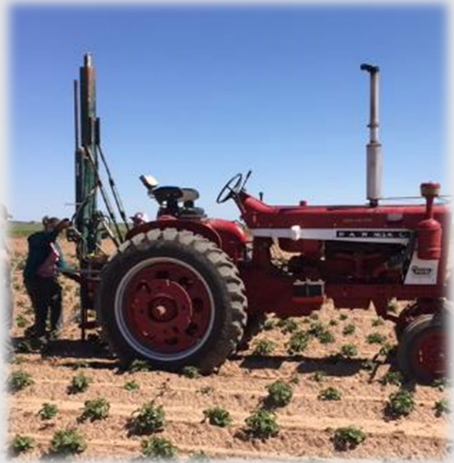
Installing neutron access tubes, 10' long X 1.5" o.d.
