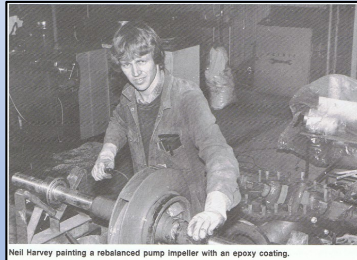
Neil Harvey painting a rebalanced pump impeller with an epoxy coating.
