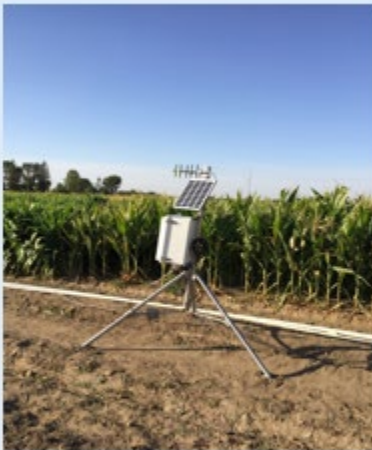
Fig. 5. Flowmeter Monitoring Station (Corn/Sorghum)
