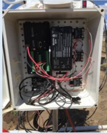
Fig. 3. Controller with Telemetry (Tomato & Lettuce)
