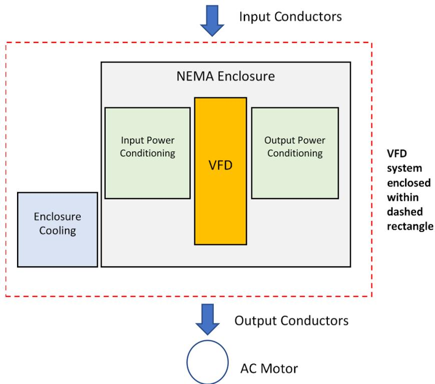
Figure 1. Major potential components of VFD systems
