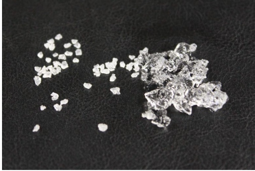
Figure 4. Comparison of dry vs. hydrated superabsorbent polymer crystals
