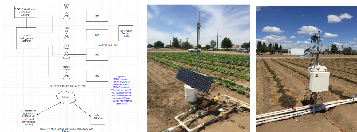
Figure -1 Block Diagram of Overall System Design for ET and Soil Sensor Based Irrigation (Left), and photos of Lettuce plot (Middle) and Tomato plot (Right).
