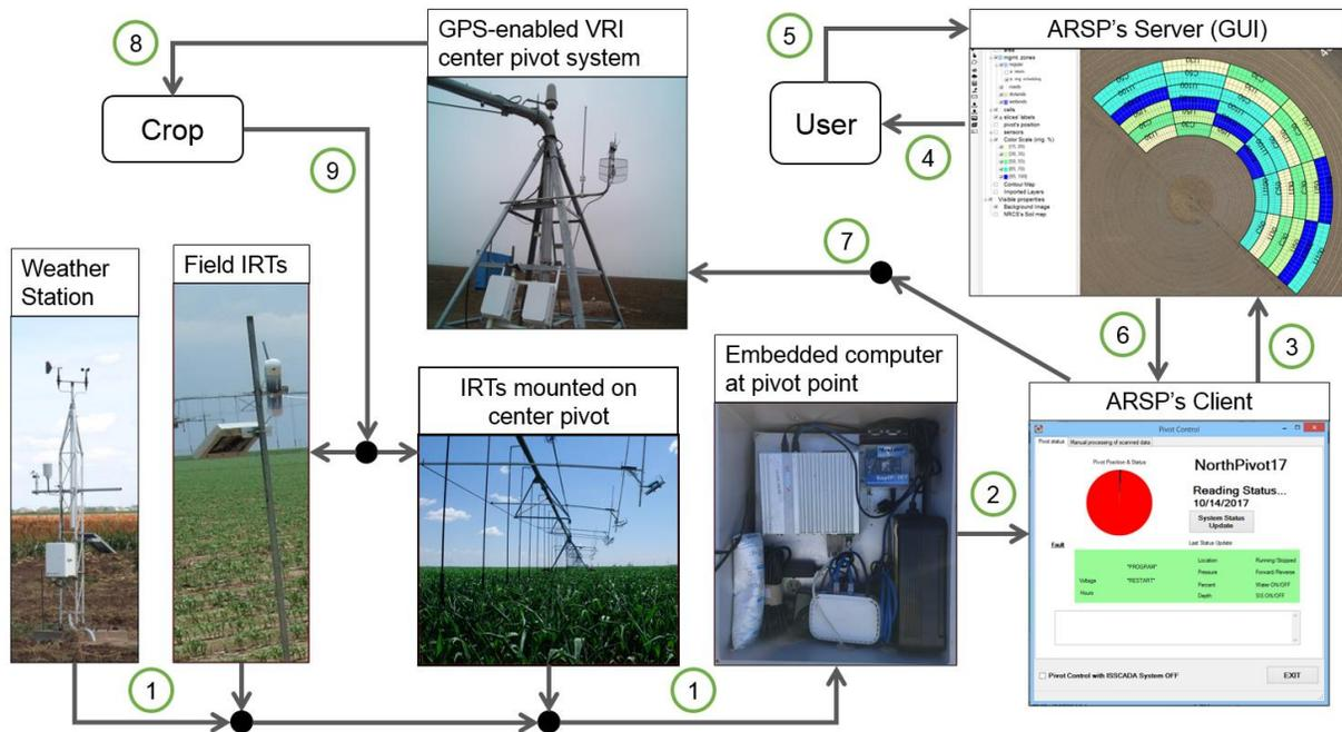
**Fig. 2. Interaction of a sensor based DSS with its user and a VRI center pivot system for the generation and application of a site specific prescription map. The process occurs through nine stages noted by numbers.**
