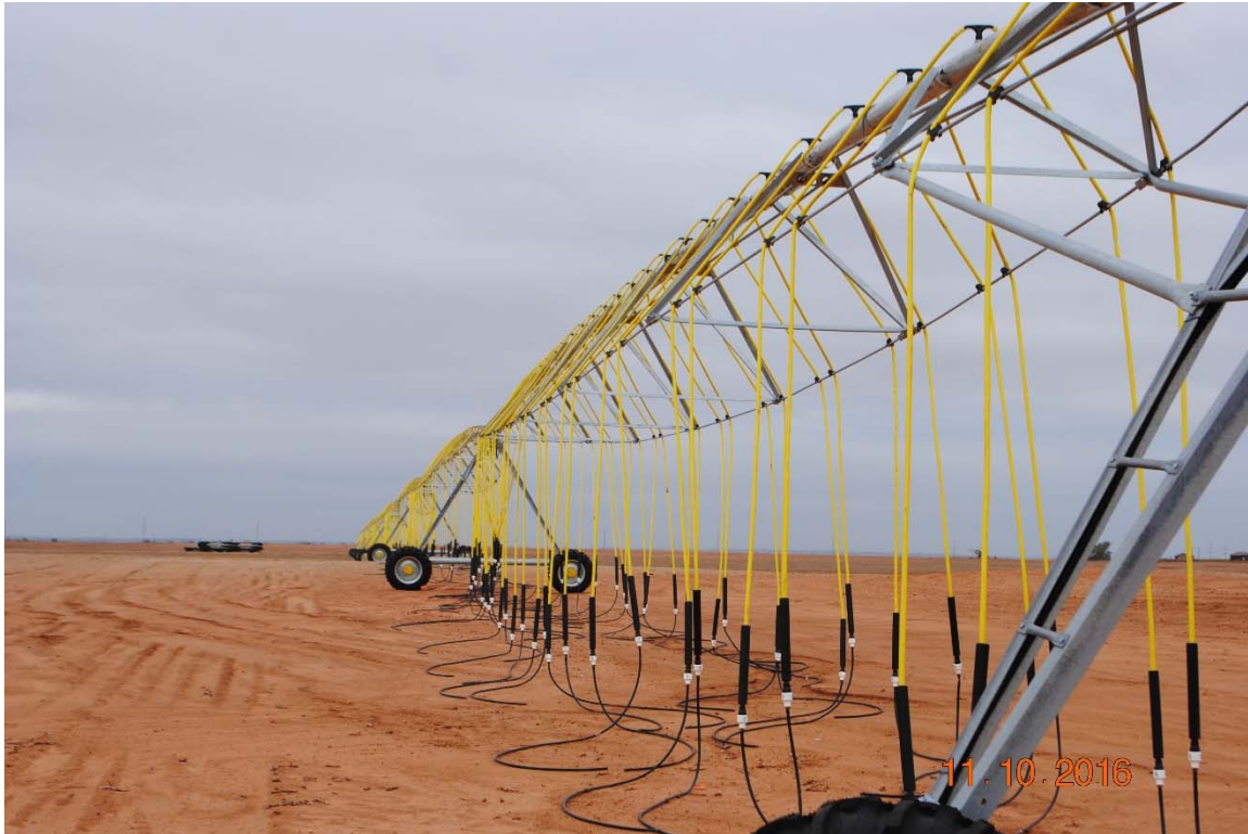
Figure 3. Drag Line System Design from the pivot mainline
