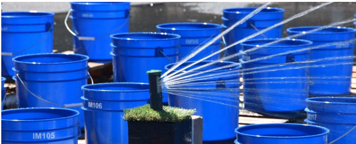
Figure 4 – Digital Sprinkler Test, Northern Water
