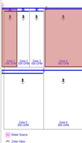
Figure 8: Before the availability of FlowControl, systems were designed to run in 3 sets when the normal 400 gpm was available from the water source. Illustration courtesy of Randi Gladwell, Clearwater Supply.
