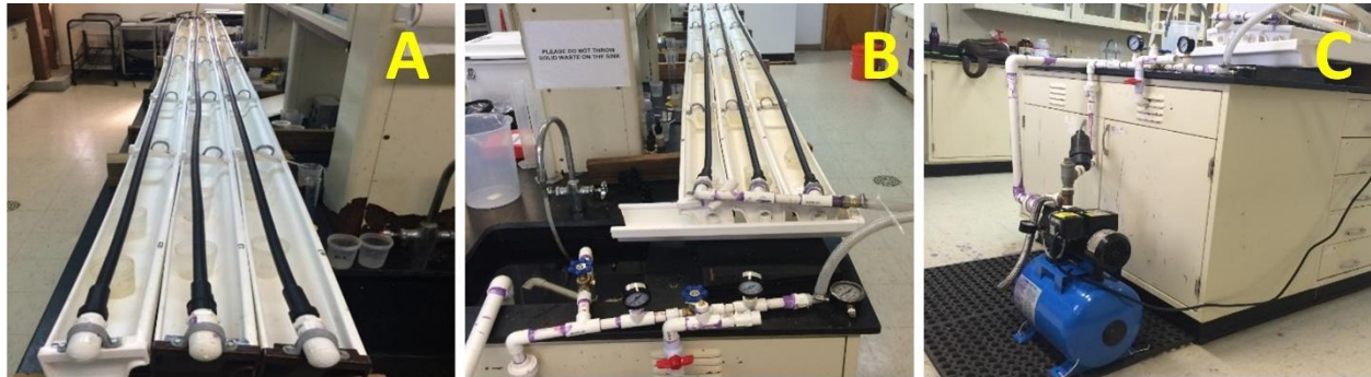
Fig. 3. Experimental module designed and installed to evaluate the effect of increasing operational pressures on drip irrigation equipment water flow. Kingshill, U.S. Virgin Islands.
