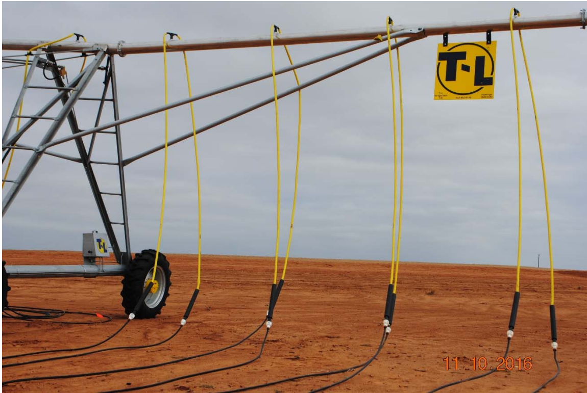
Figure 4. Drag Line System Design as with 2 drip lines per pivot drop.
