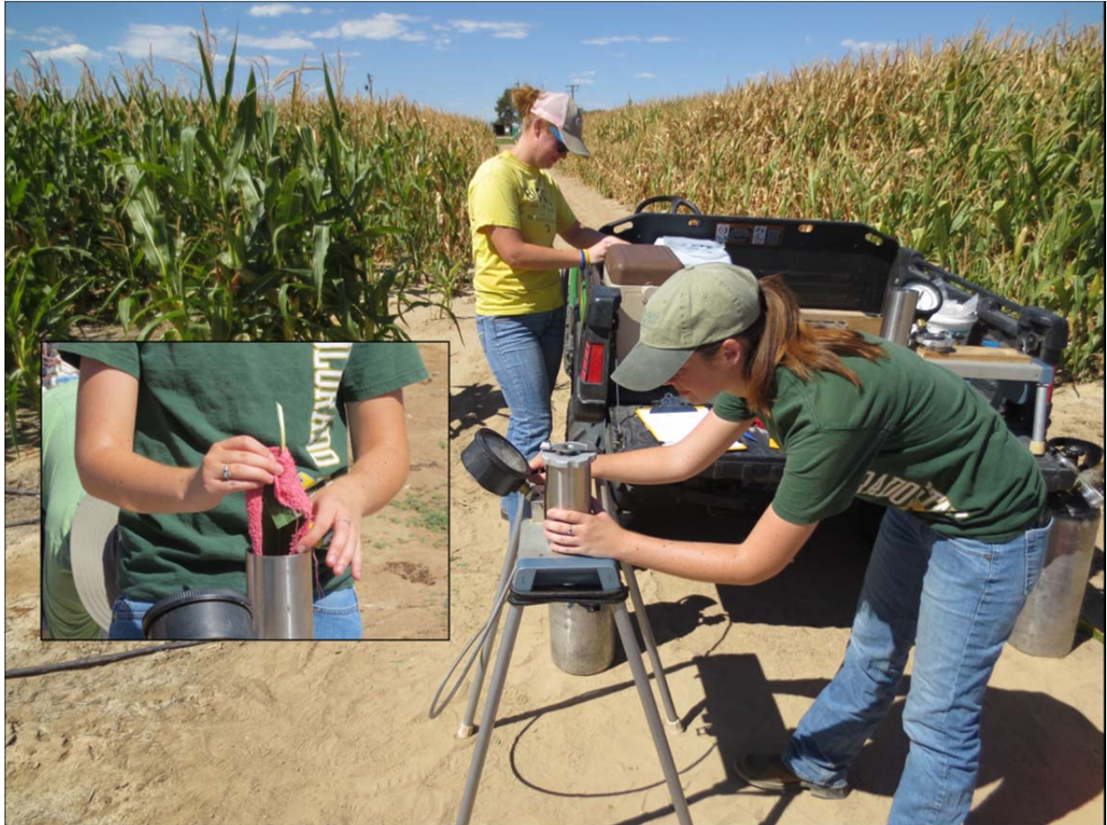
Figure 9. Midday leaf water potential ( \Psi_L ) measured with a pressure chamber. A distal portion of a leaf is cut, put in a zippered plastic bag, and transported in an insulated cooler to the pressure chamber, where it is trimmed with a razor blade, covered with a damp cloth, and placed in the chamber for measurement.
