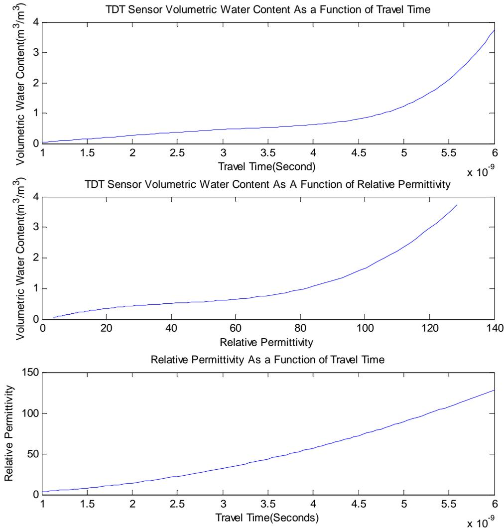
**Fig 2: MATLAB Simulation of TDT Sensor for Volumetric Water Content as a Function of Travel Time (Top), Relative Permittivity (Middle) and Relative Permittivity as a Function of Travel Time (Bottom)**
