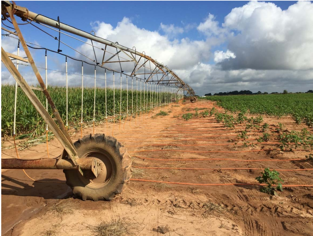
Figure 2. Drag-line system parked on end of field.
