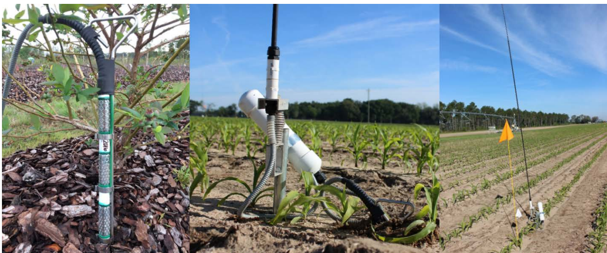
Figure 3. A UGA SSA sensor node has a low profile when installed in the field. The flexible whip antenna allows field vehicles to pass directly over the node.
