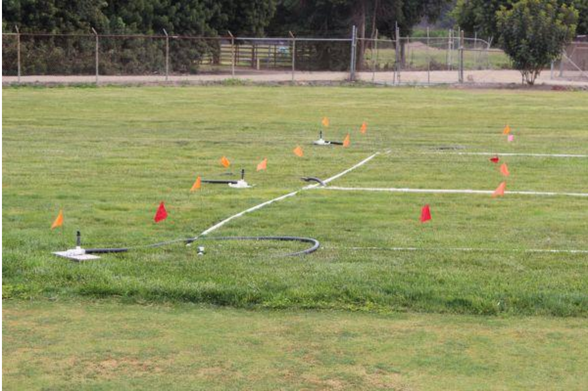
Figure 3. Sprinkler nozzles on shrub adapters mounted on movable platforms to set required nozzle spacings.
