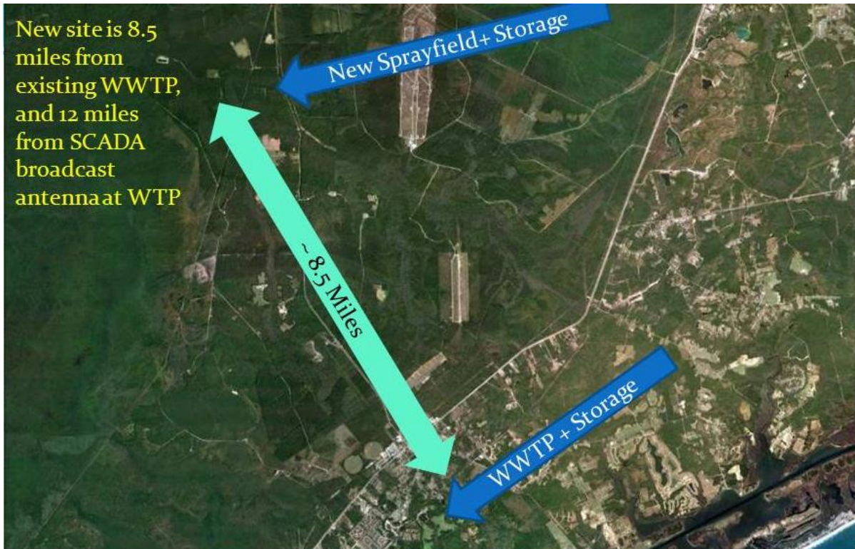
Figure 3. Expansion of SCADA Communications System for New Irrigation Site
