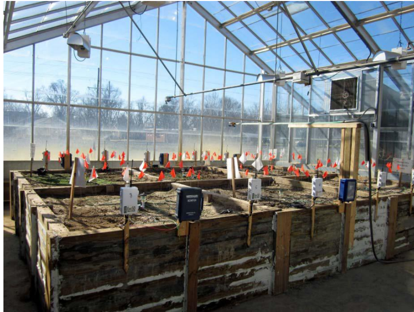
Figure 1. Six soil compartments with the sensors and data loggers installed.
