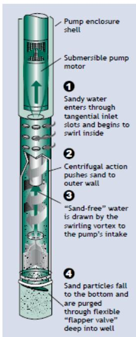
**Figure 10. A cutaway diagram of a down-hole separator.**
