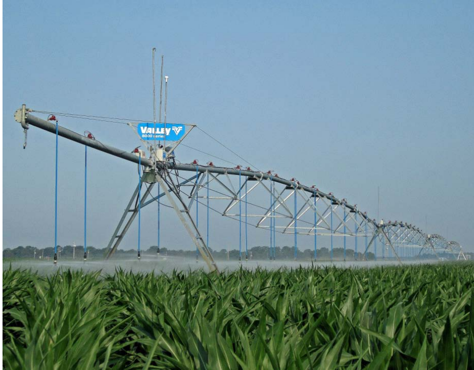
Figure 1. Four-span Valley 8000 center-pivot variable-rate irrigation system.
