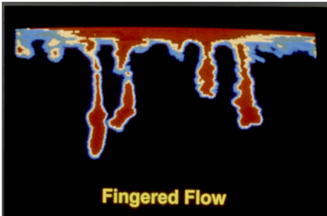
Figure 8. Preferential Flow Paths. Figure courtesy of Tammo Steenhuis, Cornell University.
