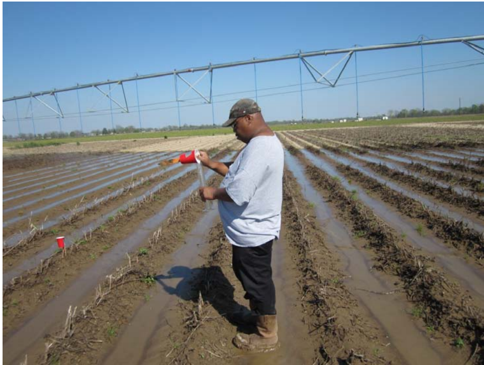
Figure 4. Water was collected and measured using a graduated cylinder.
