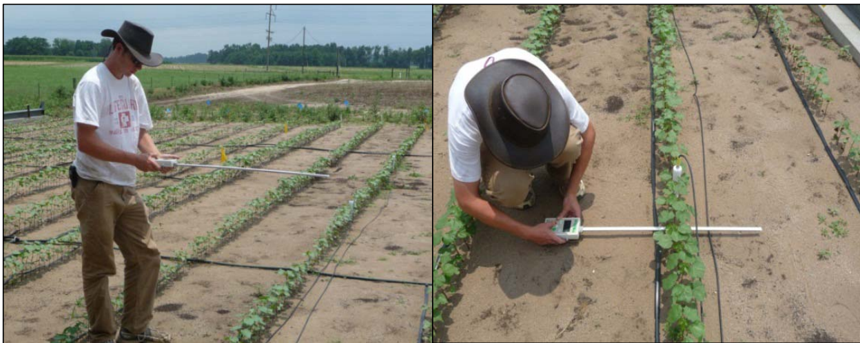
Figure 2. Measurement of PAR above (left) and PAR below (right) at the shelter plots
