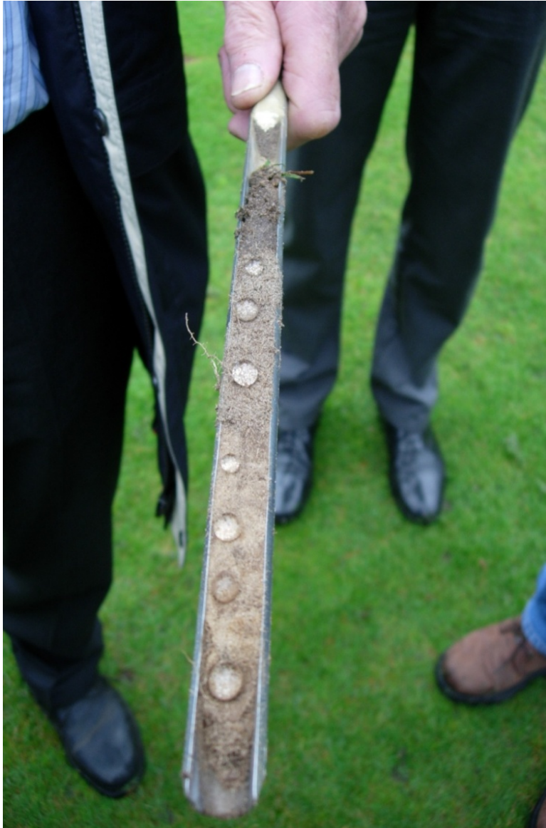
Figure 6. WDPT conducted on a soil core. Photo courtesy of Demie Moore.
