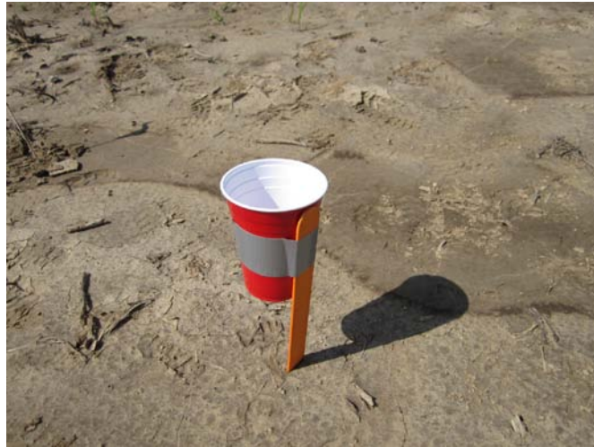
Figure 3. Plastic cup to be used as the water collector.
