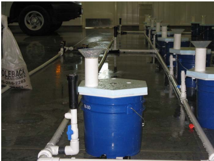
Figure 2. The sprinkler head set up for catch can tips at ground level.
