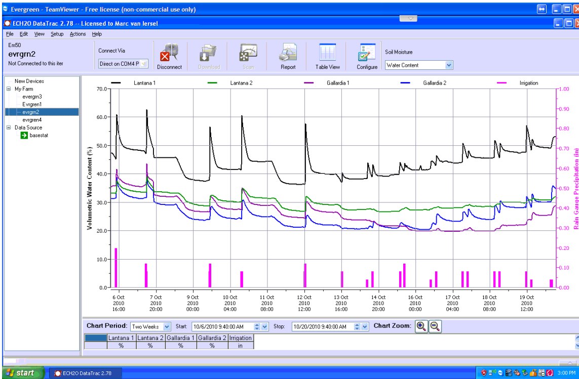
Figure 2. Screenshot showing the DataTrac graphic user interface. The four lines show substrate water content of two containerized lantana (green and black, plants in #2 containers)) and two gaillardia plants (purple and blue, #1 containers). Pink bars indicate rainfall or irrigation events. Irrigation was changed from once daily to twice daily on October 14.
