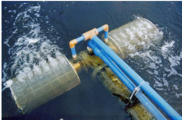
Figure 1: Pump intake screen
