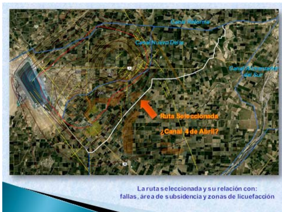
Figure 12. Route of new April 4 canal, showing faults, subsidence, and liquefaction zones.
