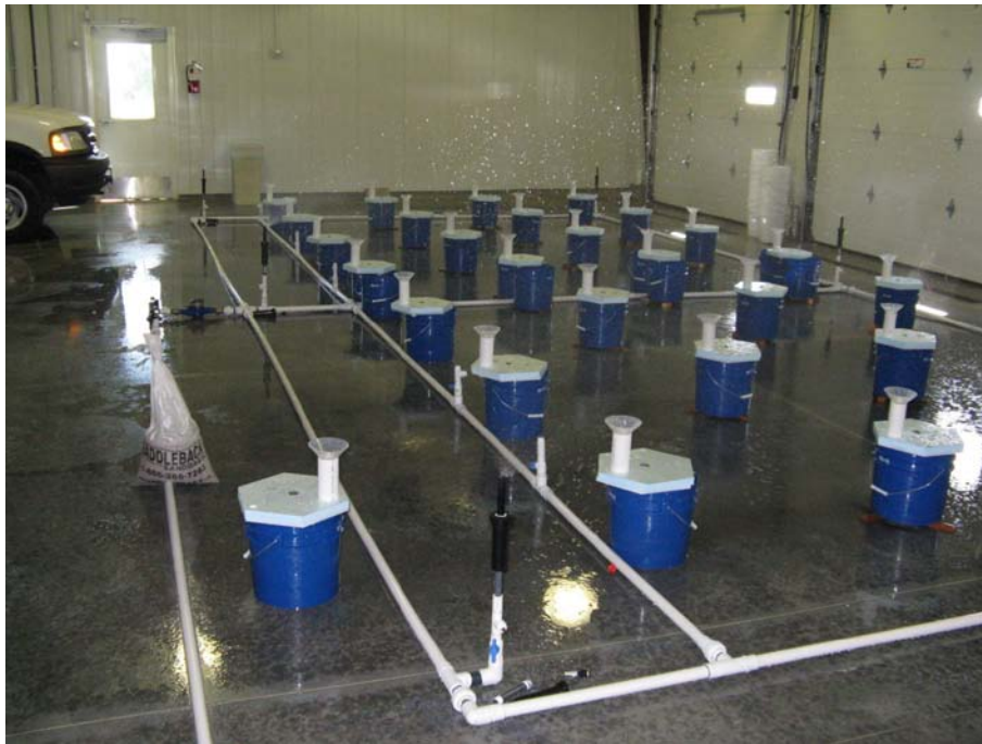
Figure 1. The indoor irrigation system set up for catch can rims at ground level. Each catch can support was shimmed so level was maintained from center to garage doors.
