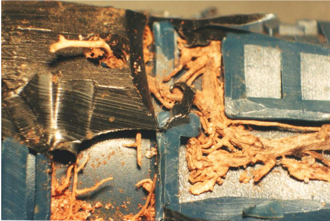
Figure 6. Single coffee plant root entering an emitter can enlarge into a large root mass once inside the emitter and dripline. Photo courtesy of Rubens Duarte Coelho, University of Sao Paulo, ESALQ / Brazil.
