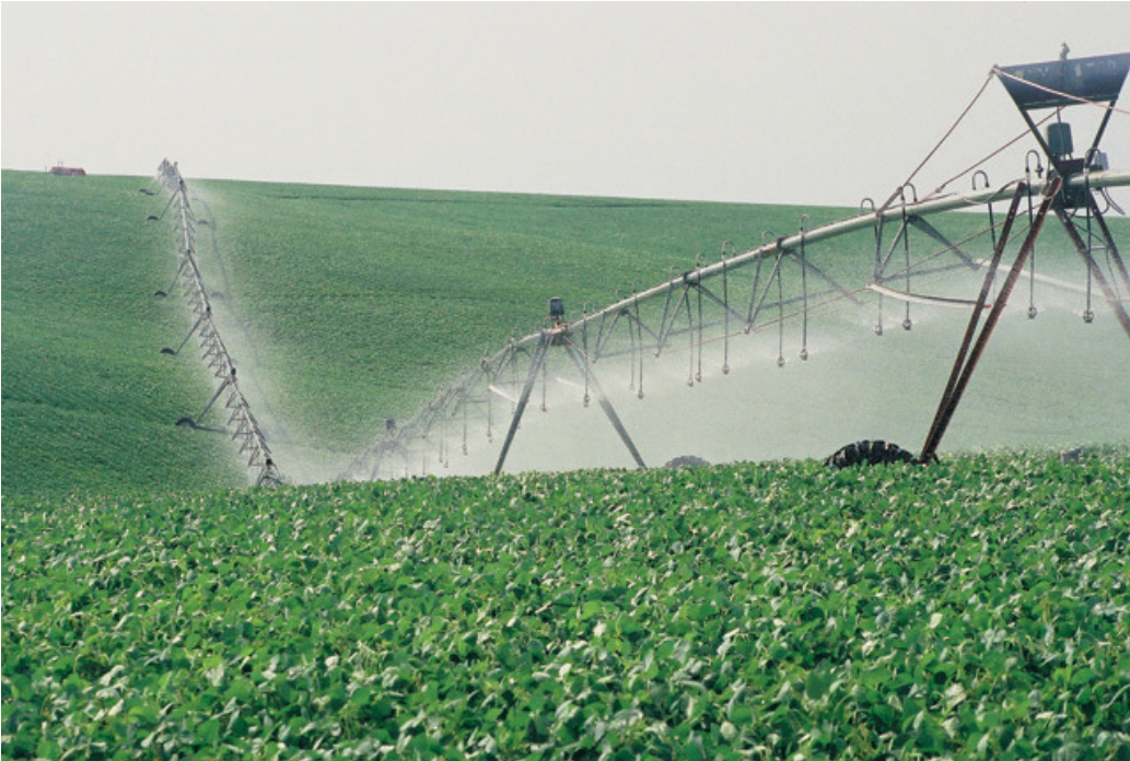
Fig. 1b: A photo showing a center pivot operating across varying field elevations.
