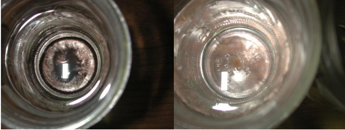
Figure 2. Jars containing Mn at 0.15 g material/gal of irrigation water, both at 0.125% H 2 O 2 concentration. The pH of the container on the left was 7.6; the pH of the container on the right was 6.5.
