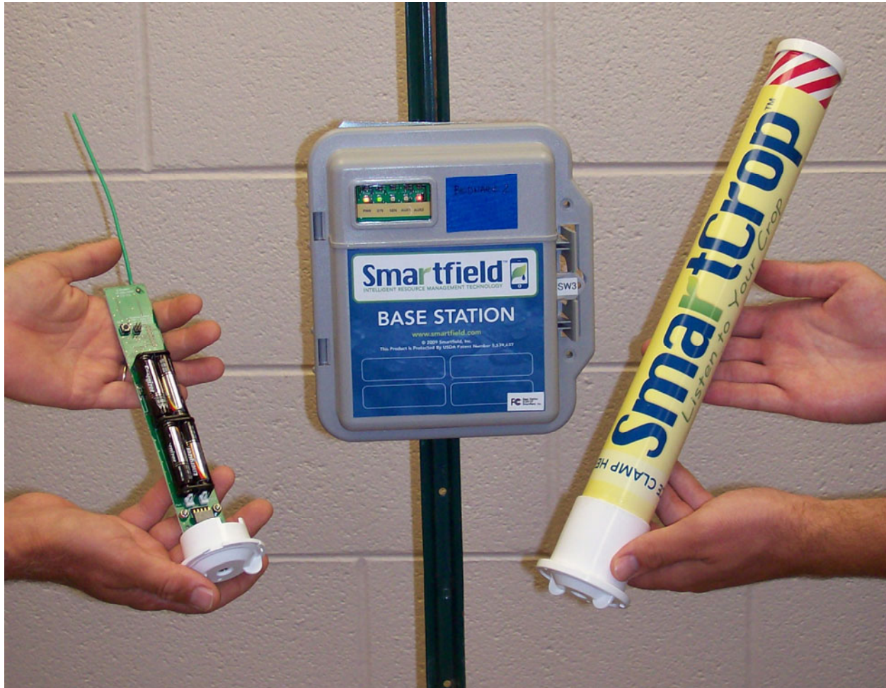
Figure 2. Low-cost wireless infrared thermometry system for research/production use.
