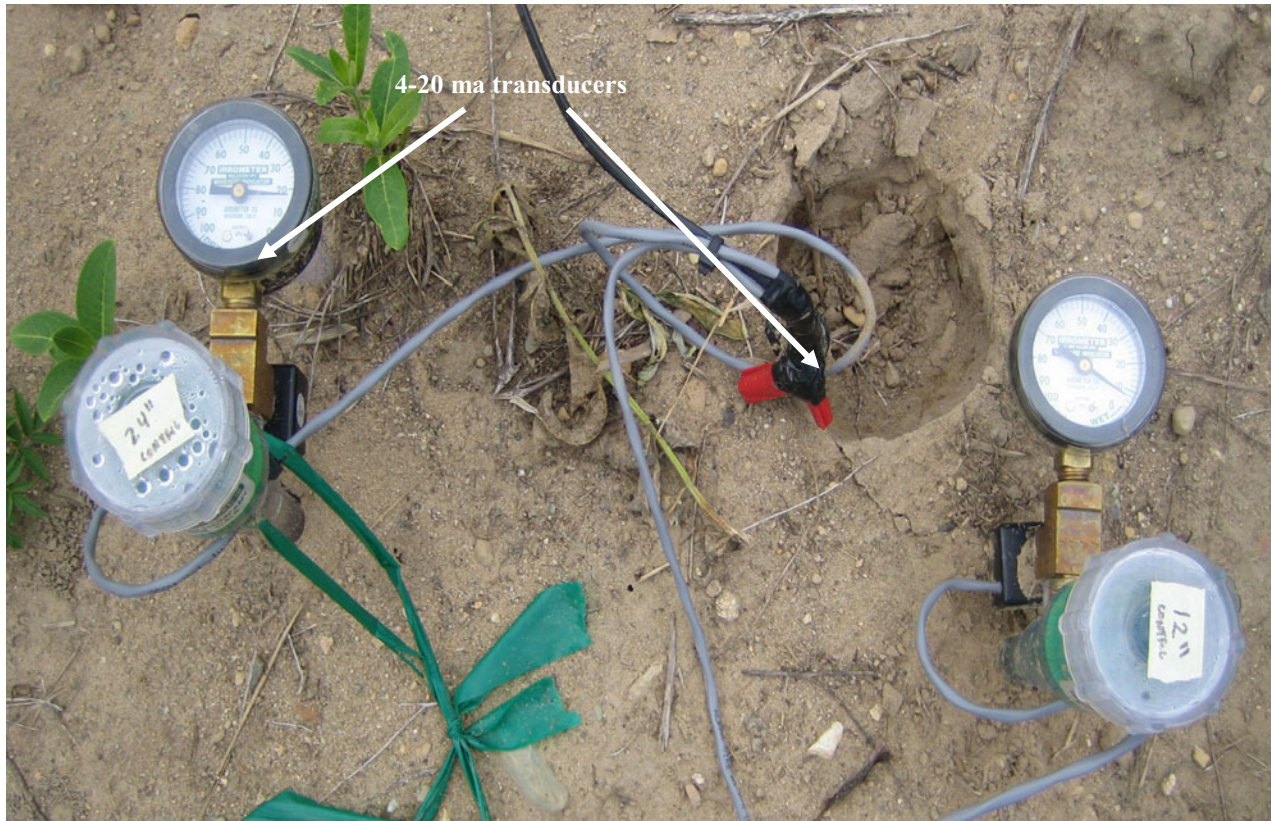
Figure 3: Tensiometers (30 cm and 60 cm) installed in the ground. Each tensiometer had a vacuum gauge and 4-20 ma transducer wired to the multiplexer.
