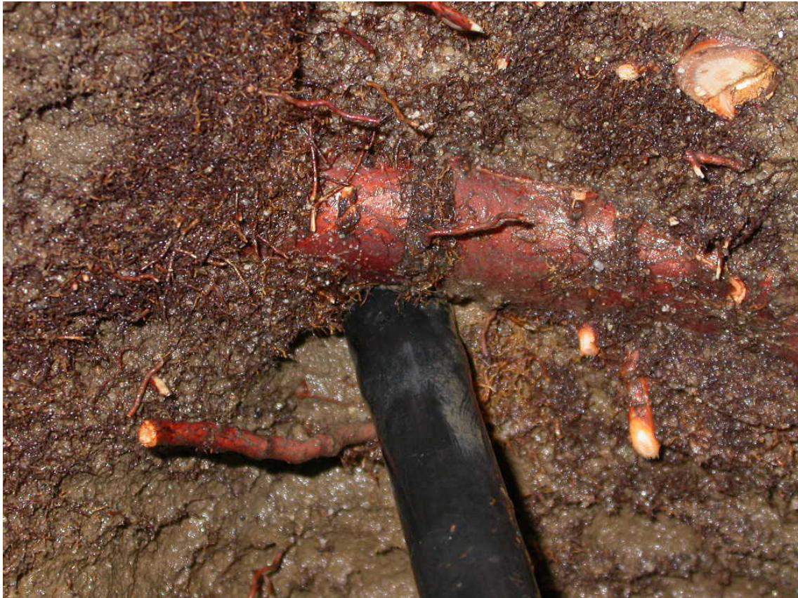
Figure 7. Subsurface dripline pinched by peach tree root in California, USA. Photo courtesy of T. Trout, USDA-ARS, Parlier, California.
