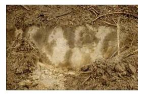
Water drop penetration in wettable and repellent soil. Preferential flow in repellent soil. Courtesy Alterra,
