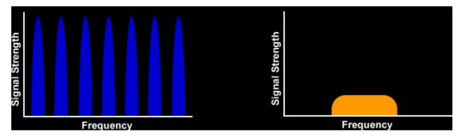
The FCC allows two methods for building spread spectrum radios: Frequency Hopping Spread Spectrum (FHSS) or Direct Sequence Spread Spectrum (DSSS)
